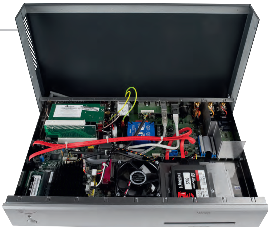
The internal hard disk houses the operating system and buffers ripping data. The fan in the center is absolutely inaudible.
